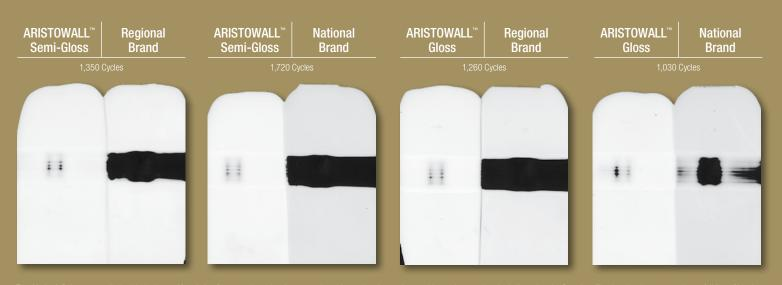
Test Method: Paints are applied to black charts. After drying for seven days, the charts are placed in an abrasion testing machine and stopped at the indicated cycle. Complete film deterioration occurs when a full line of black background is exposed.
