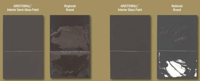
Test Method: Paints are applied to black and white charts and allowed to dry for 24 hours. The charts are then cut and folded over each other. A weight is then placed on them to force the painted surfaces together. After 24 hours, the face-to-face charts are pulled apart to see if the dried paint stuck together.
